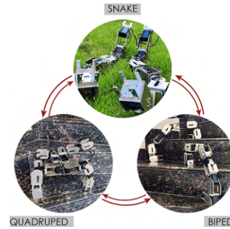
Fig. 1. Illustration of various mobility modes of ReQuBiS.
